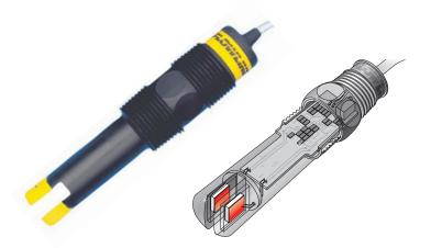
CSA approved for hazardous environments, the intrinsically safe ultrasonic point level switch provides reliable liquid level detection of chemical, solvent, hydrocarbon and petroleum based liquids with a 1A relay output. Media examples include fuel, acetone and hydrochloric acid. The submersible polypropylene or PFA liquid level sensor is universally mounted through the tank wall or inside the tank as a high level alarm or low level alarm.
